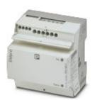
Multi-functional energy measuring device without display with direct Rogowski connection and integrated Modbus/TCP interface for measuring electrical parameters in low-voltage installations up to 690 V.
