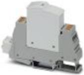
Type 2/3 surge protection, consisting of protective plug and base element with Push-in connection. For single-phase power supply network with integrated status indicator and remote signaling. Nominal voltage: 230 V AC/DC
